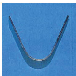
No crack was formed even in 180-degree bending test.
